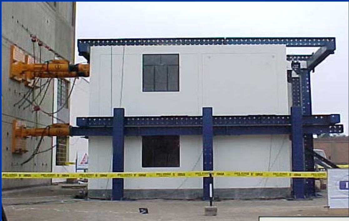
Hydraulic jacks applying lateral forces
