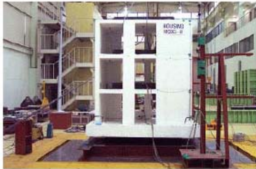
Figure 5.4.16 A 1/3 scale model on a shaking table
