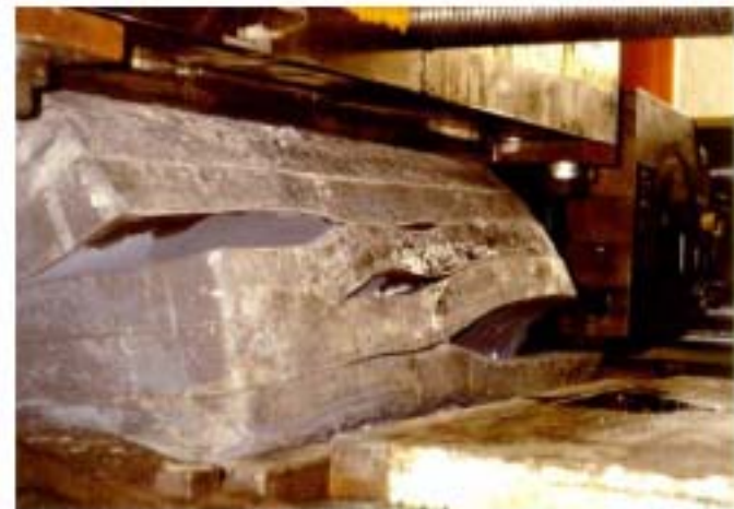
Fig. 5.23.c. Occurrence of the first cracks between the layers of the bearing
