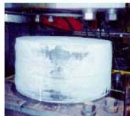
Figure 5.4.6 LRB chilled to -28^{\circ}\text{C}
