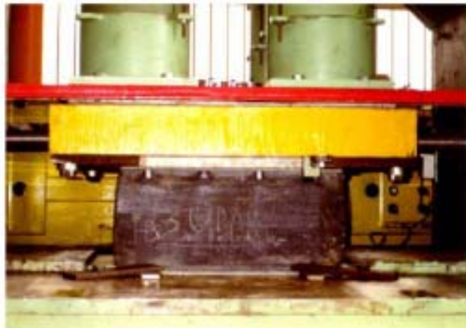
Fig. 5.5. Bearing Placed on a Press, prior to testing
