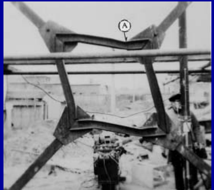
Energy dissipaters using steel (1979) full scale tests
