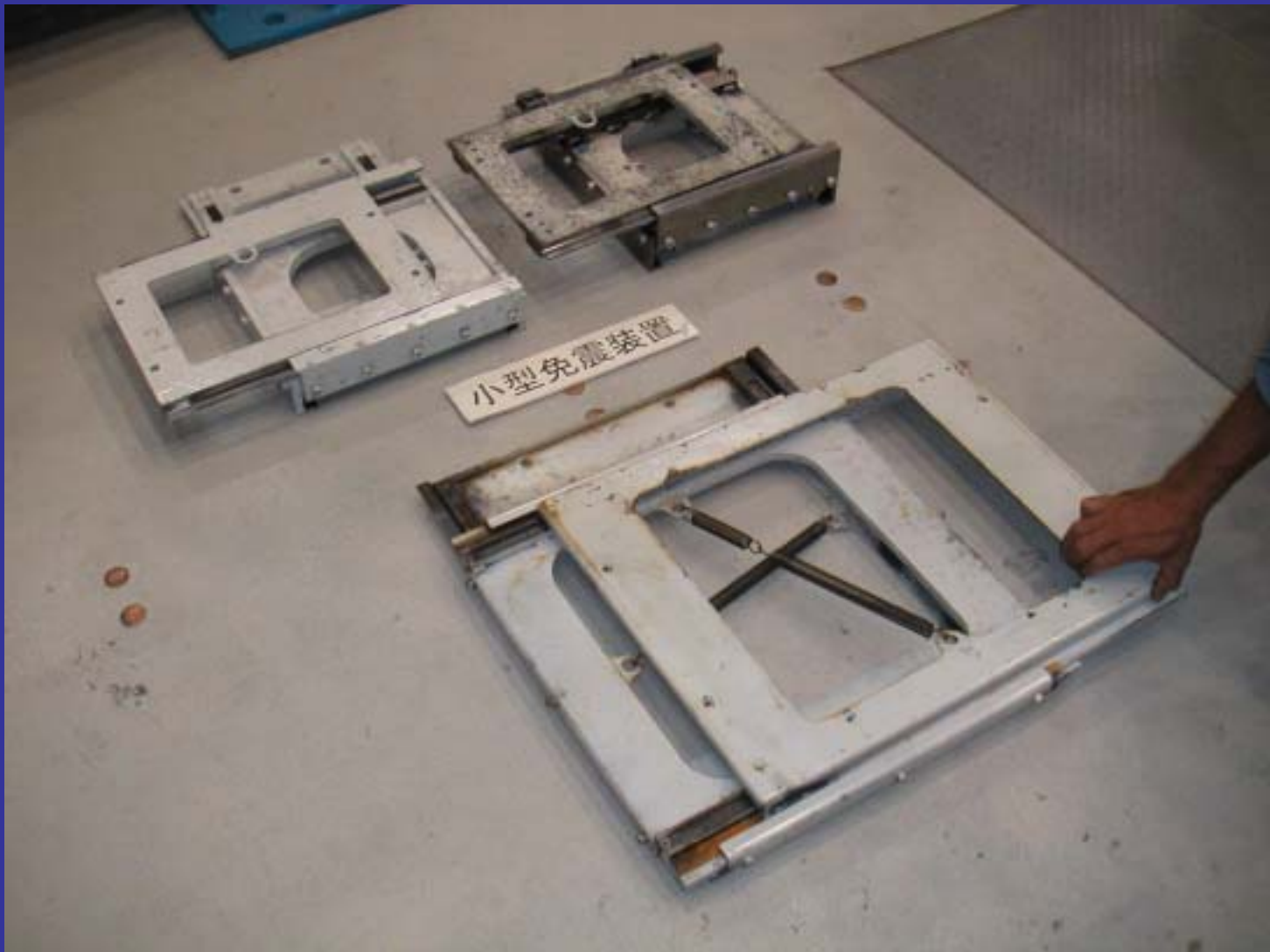
Isolator for the shaking table and prototype isolators (upper two)
