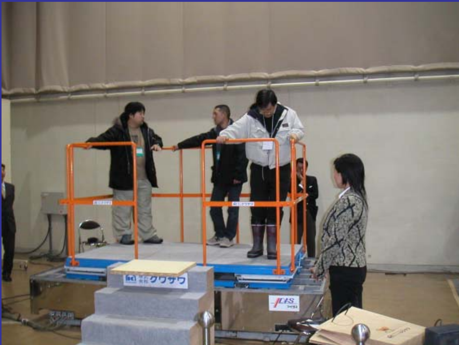
Demonstration of isolators using a shaking table
