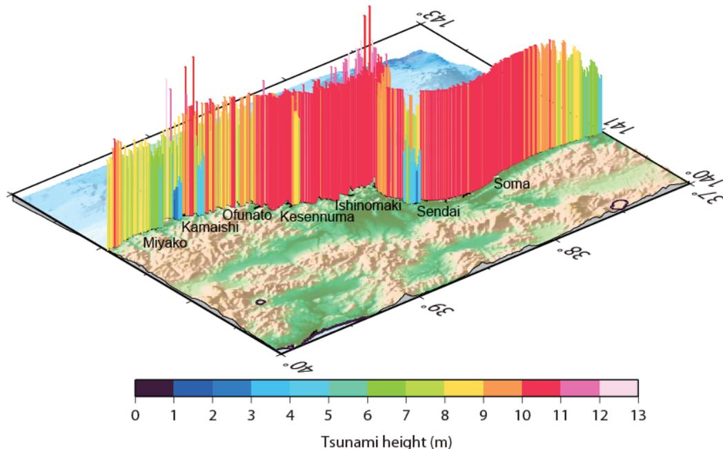
Fig. 4.4-6 Simulated tsunami heights along the coasts from southern part of Iwate to Fukushima prefectures. The used tsunami source model is based on Fujii *et al.* (2011) 4-8).
