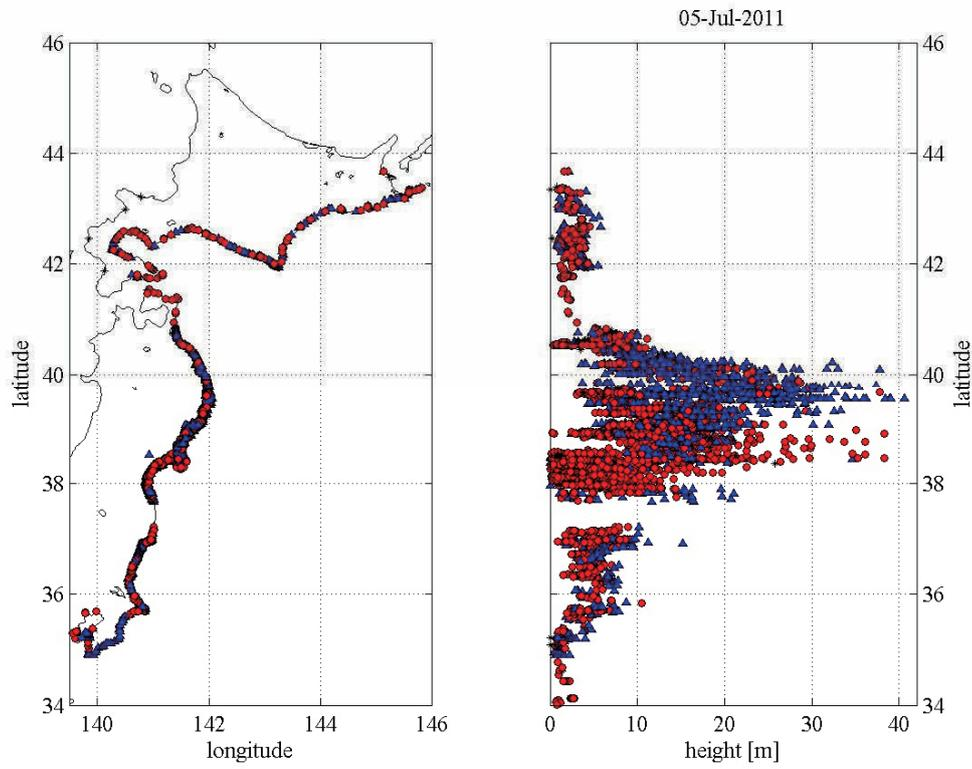
Fig. 4.4-2 Distribution of measured tsunami heights by the field surveys<sup>4-7</sup>): Red circles and blue triangles indicate inundation heights and runup heights, respectively.
