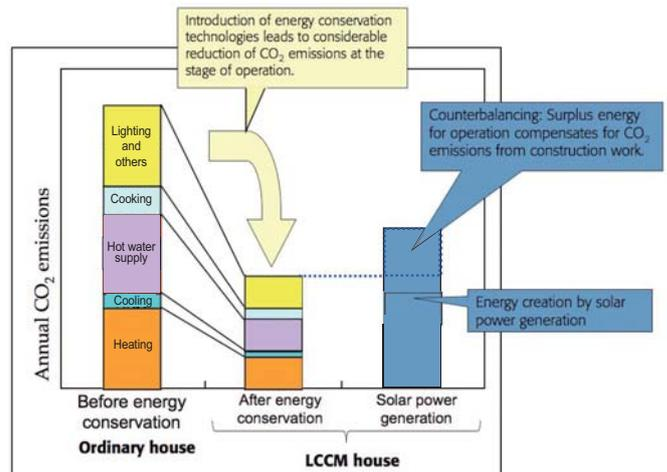
Figure 6: Energy Balance of the LCCM House
