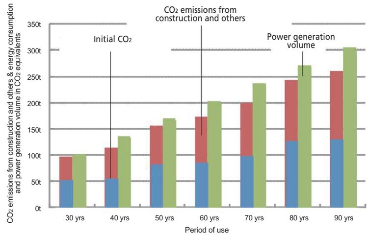
Figure 8: Trend in CO<sub>2</sub> Emissions and Power Generation Volume (Under the condition with the use of a solar thermal hot water system with natural refrigerant and with the unit CO<sub>2</sub> emissions of 0.418 kg-CO<sub>2</sub>/kWh on average for all power sources)
