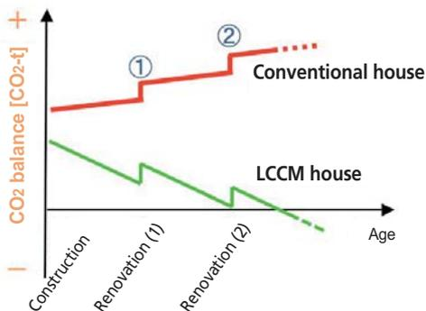
Figure 7: Schematic of CO<sub>2</sub> Balance throughout the Life Cycle
