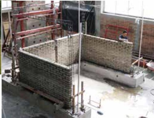
A framework masonry test structure using the soil-cement method under construction at Central American University
