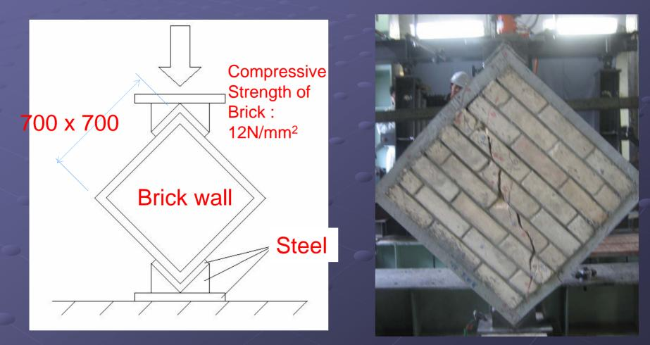
Parametric experimental study to examine effect of strengthening methods on improvement of in-plane behavior of confined brick masonry wall
