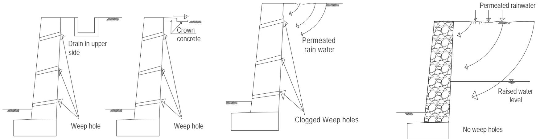
Weep holes, Exuded water and Drainage conditions
