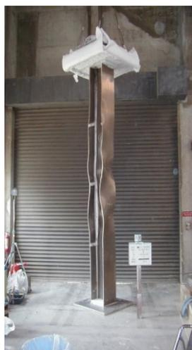
A column sample after a test using the vertical furnace for columns
