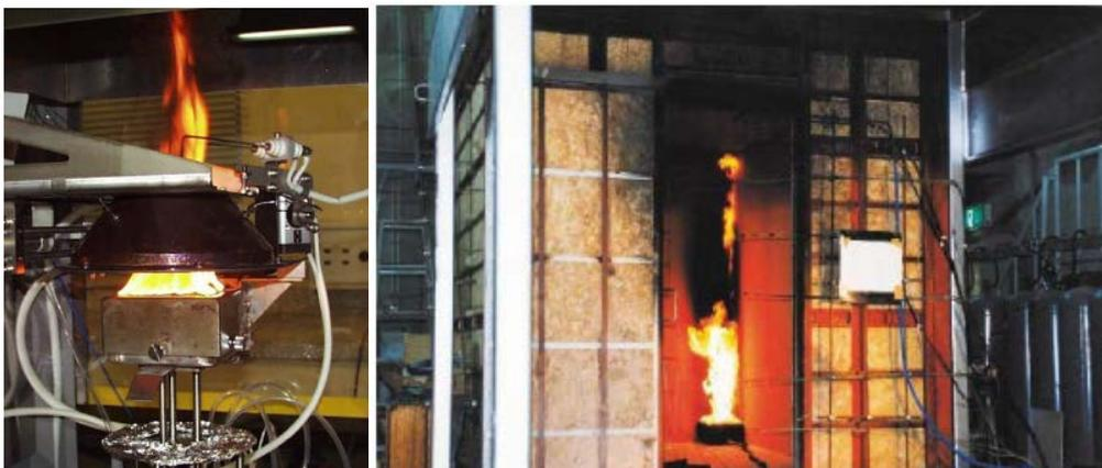
Examples of heat release and smoke production test using cone calorimeter (ISO5660), and full scale room corner test for surface products (ISO9705)
