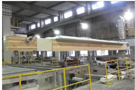
A beam sample before a test using the horizontal furnace
