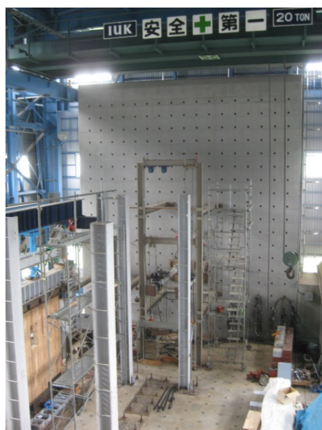
<Reaction wall and slab>
