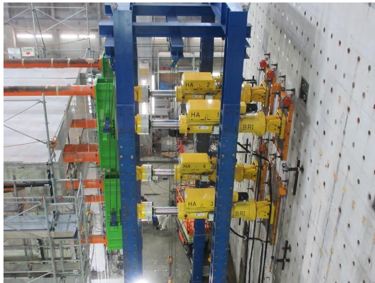
Loading test with hybrid hydraulic actuators (Four actuators are controlled at the same time)
