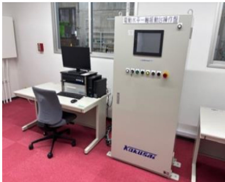
Shaking table excitation control device
