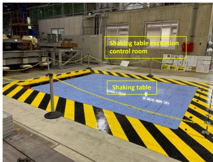
Overall view of the shaking table testing area
