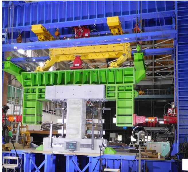
Experiment with column specimen under anti-symmetric moment condition
