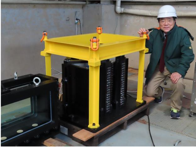
Shear box for the centrifuge
