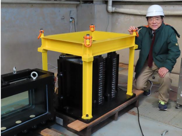
Shear box for the centrifuge
