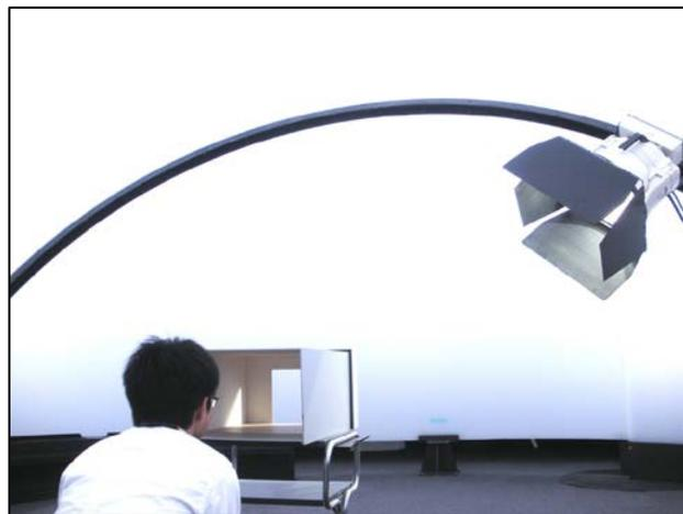
Subjective experiment using scale model under the artificial sky
