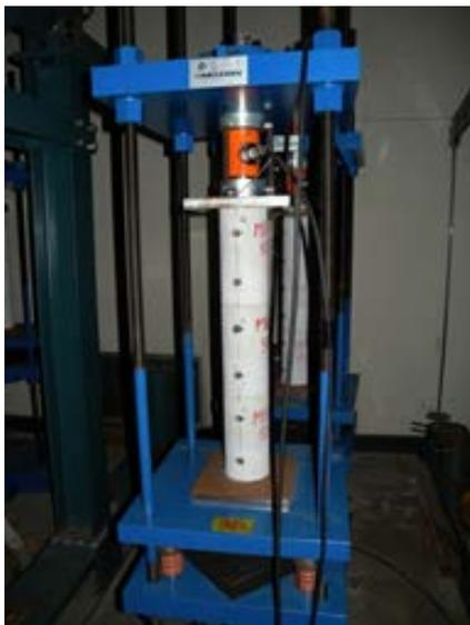
Creep Compression Test of Cylindrical
