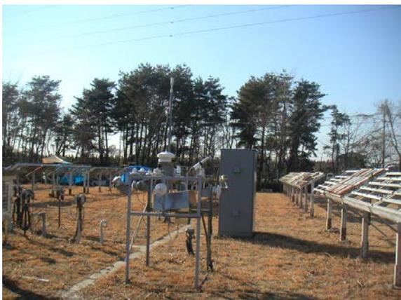
weather factors after making reference to those of gained in meteorological office to prove they are not inadequate. And we also manage the thermo-data and others of materials under Outdoor Exposure Test, for the quantification of degrader factors on the material's or parts' durability.
