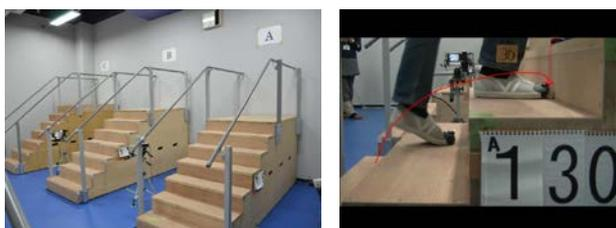
(Photo 2) Experiment on an appropriate height of rise of a step
