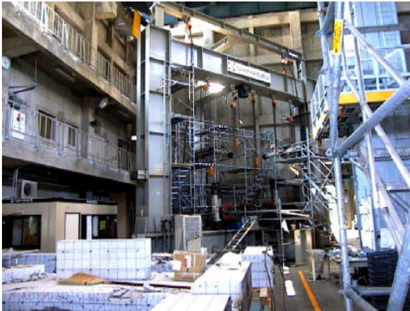
Reaction frame in Building Research Institute , Tsukuba, Japan
