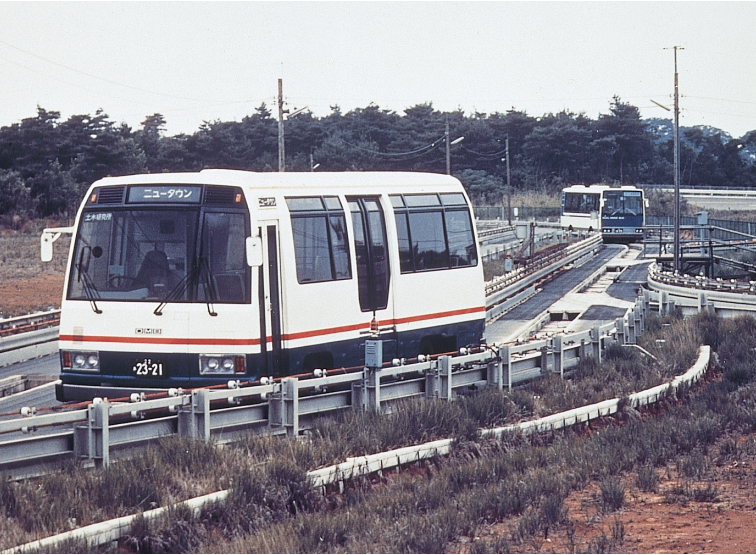
3.新道路交通システムの開発 ワンマンバスとガイドウェイバスの両方の機能を備えたデュアルモードバスシステム Development of the new road transport system The dual-mode bus system consists of buses that can not only run automatically on guideways but also be driven by a driver on ordinary roads.
