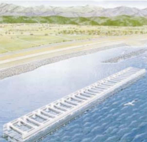
22. 海洋利用空間の創成・保全技術の開発 多目的海洋利用空間を創出するための消波構造物（下新川海岸） Development of technology for creating and preserving marine space Wave-absorbing structures, such as the one shown here along the coast at Shimonikawa, create space by the shoreline that can be used for many purposes.
